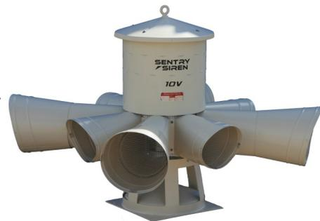
and with a 10 HP, continuous duty motor pushing its aluminum rotor, this siren produces 115 dB(c) @ 100 ft. continuously. The 10V utilizes staged horn projectors, 4 long and 4 short. This design helps to spread sound over the coverage area more evenly, balancing the need for short distance penetration with long distance throw.
